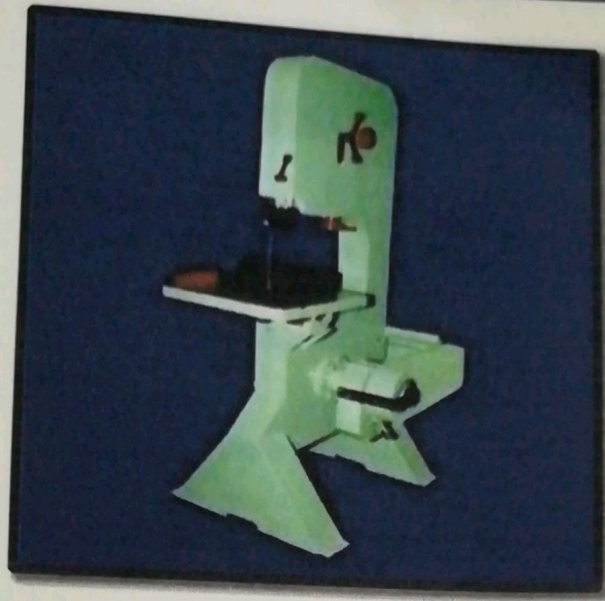
Fig 3.1.6 Band hacksaw machine
